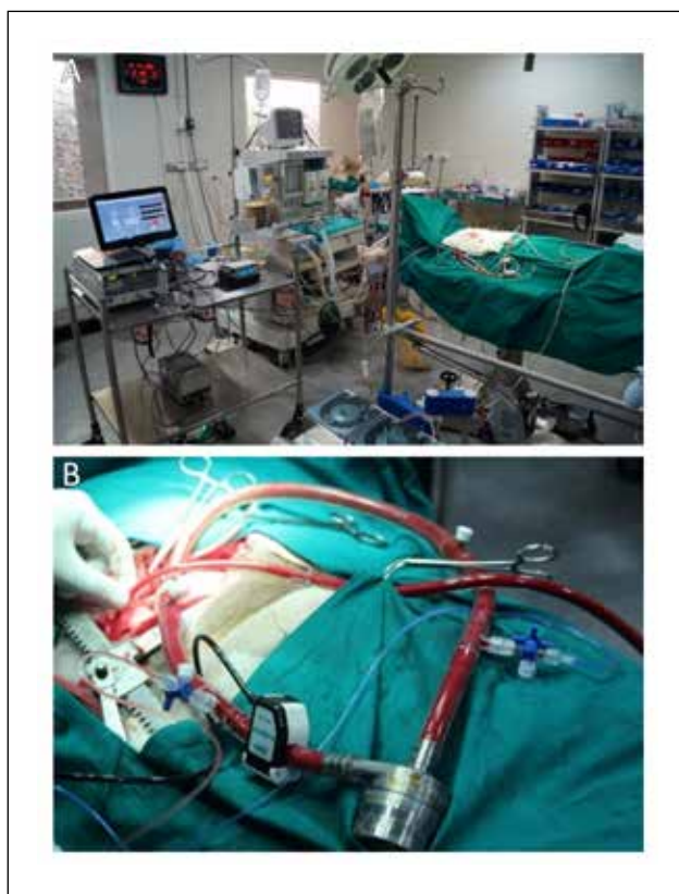
Figure 37. A. Chitra pLVAD ex vivo evaluation setup B. Ex vivo connected Chitra pLVAD
