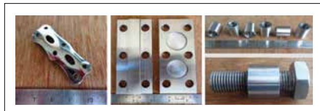
Figure 55. Completed the machining of Ti 6Al-4V implant prototype and SS stress relief fixture for the TRC project 8221 of AIO Lab
