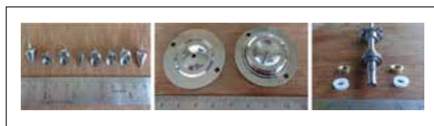
Figure 53. Completed the machining of Ti CP-2 top thrust magnet holders and Ti CP-2 magnet holder caps for the pLVAD project P8123 of ECD Lab, SS ASD occluder shaping mould for the TRC project 8150 of AIO Lab and Delrin and Brass spacers for the ball screw mechanism of Raman confocal microscope for the TDF project 6244 of CAF Lab.
