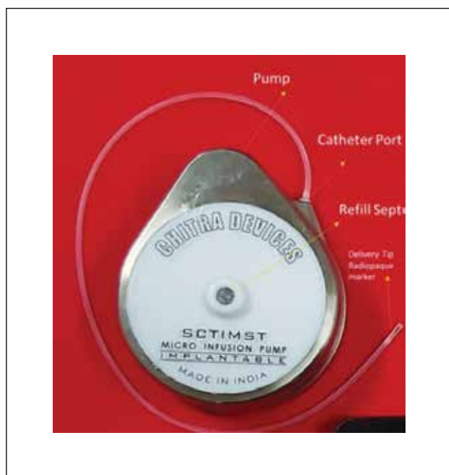
Figure 38. Implantable micro infusion pump prototype with catheter
