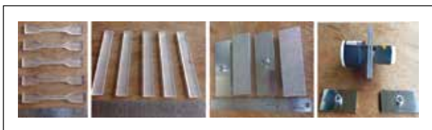
Figure 56. Completed the machining of acrylic test samples (ISO 527 & ISO 178) for PMD and SS tensile grips for the TDF project 6244 of CAF
