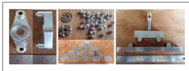
Figure 52. Completed the fabrication of aluminium bearing holder for the Division of Dental Products, Ti CP-2 IIP CAM bottoms, CAM top covers, rollers and needle stoppers for the TRC project P8138 of ECD Lab and Four point-bending fixture for the TRC Project 8221 of AIO lab.
