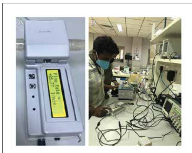
Figure 39. A. Prototype of Blood flow meter manufactured by industrial partner and B. testing of industrial unit
