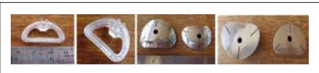
Figure 57. Completed the machining of polycarbonate annuloplasty ring holders and SS marker fixtures - sizes 24, 26 and 28 for the TRC Project 8128 of AIO Lab
