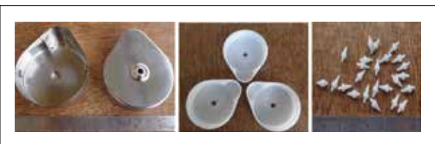
Figure 59. Completed the fabrication of Ti-6Al-4V IIP bottom casings, Delrin IIP Bottom casings and Delrin IIP Tube connectors for the TRC Project 8138 of ECD Lab.
