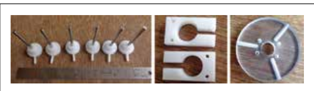
Figure 60. Completed the fabrication of Pusher System for the TRC Project 8150 of AIO Lab, Polypropylene LVDT clamp and Polycarbonate LVDT support disc for the TRC Project 8221 of AIO Lab.
