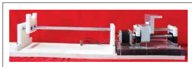
Figure 54. Completed the machining of Pushability test setup for ASG Delivery system, for the TRC project 8124 of AIO Lab
