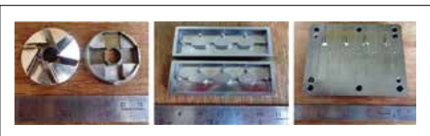
Figure 58. Completed the machining of pLVAD impeller for the TRC Project 8123 of ECD Lab, SS mould for cell culture activities for the TDF Project 8198 of DEP Lab, SS contact strip mould for the TRC project 8132 of MEI Lab
